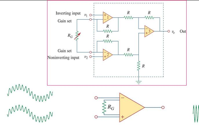
Small differential signals riding on larger common-mode signals
