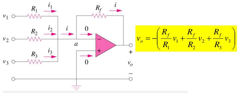
**Q:** Is it possible to construct a non-inverting summing amp?
